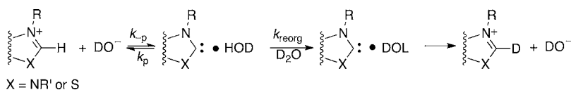
Scheme 4. Mechanism for Deuterioxide-Catalyzed Azolium Ion H/D-Exchange
